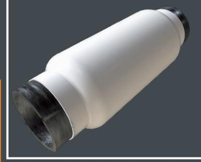
Flame Spray Polypropylene (FSPP) technologies are particularly useful with custom pieces, bends, buckle arrestors etc., items whose shapes are difficult to coat. Powder is carried in a stream of air and is fed into the center of an annular combustion flame where it is heated. A second outer annular nozzle feeds a stream of air, around the powder stream, which accelerates the spray particles toward the substrate and prevents burning of the powder.
